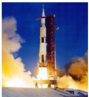
As rockets consume propellants, the tankage that originally held the fuel and oxidizer becomes dead weight. It soon becomes advantageous to discard as much of this weight as possible, which is why rockets are built with stages.
