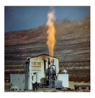
Kiwi A nuclear rocket engine test. (Los Alamos National Laboratory)
