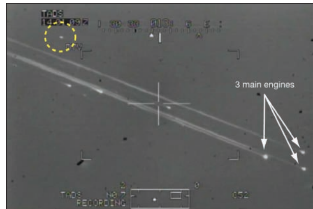
Image is from the Apache video. Dotted circle indicates area where the crew module debris was last visible. The three points in the lower right are the orbiter's three main engines. The forward fuselage and crew module fragmented into pieces quickly and became too small to detect by ground-based video. At approximately GMT 14:35:00, the crew remains and the majority of the crew module debris completed the free fall to the ground.
