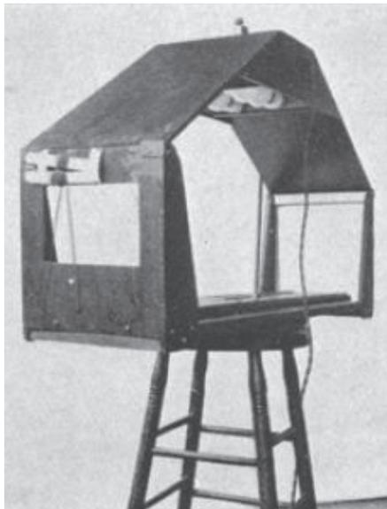
**Depth perception** - The modification to the depth perception tester pictured here kept applicants from looking over the top and also reduced glare and removed shadows from within the apparatus.
